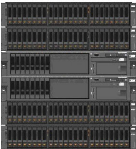
Figure 3. A GSS Model 24 configuration with 1.2 TB 2.5-inch 10k rpm 6 Gbps SAS HDDs
